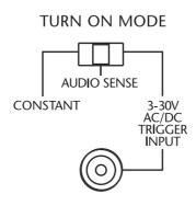
**Constant** - The auto turn-on circuitry is off. The front panel master power switch operates the amplifier. In is "On", out is "Off".
